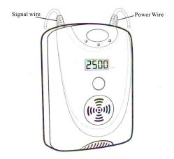
Signal wire is for relay output, black wire COM, pink wire for NC and blue wire for NO.
